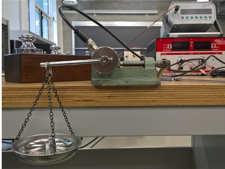
Figure 2.10: Torque-meter calibration, set up
