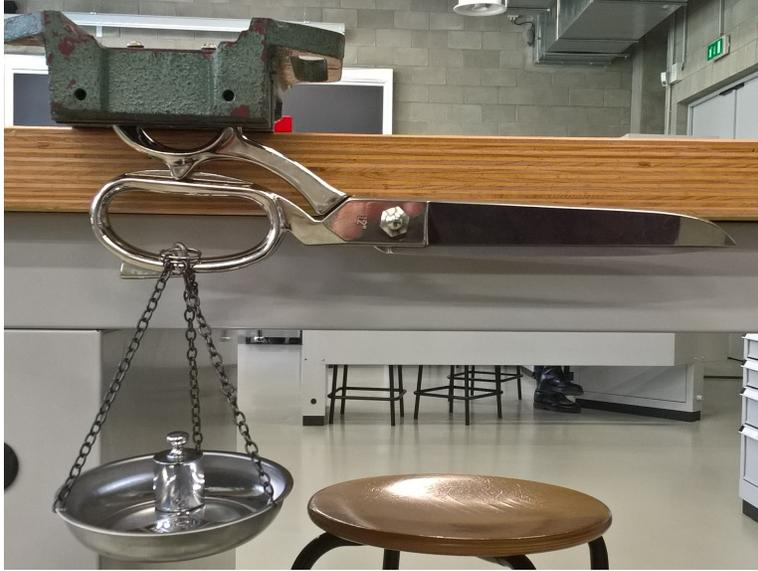
Figure 2.4: Static friction evaluation
