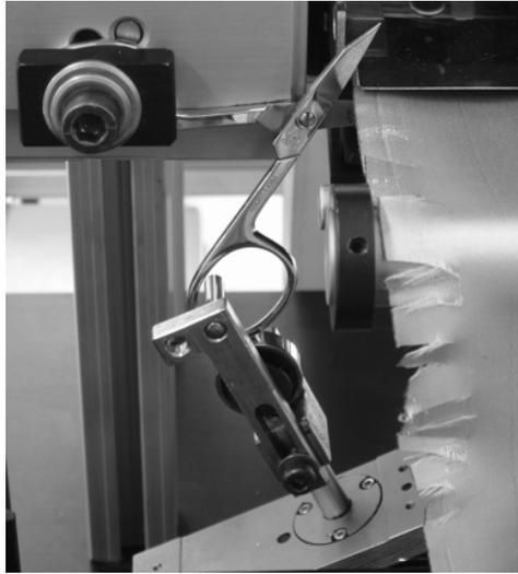
Figure 1.11: Scissors clamping and actuation mechanism
