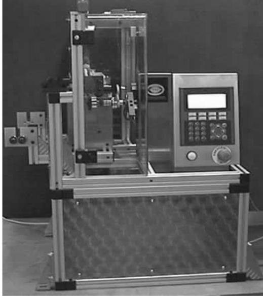
Figure 1.7: Scissors cutting performance test machine, CATRA
